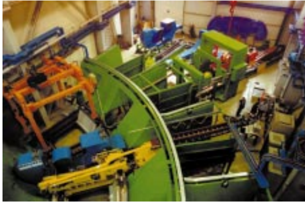
Figure 6. Divertor remote handling test platform, showing the cassette toroidal mover in remote operation.
