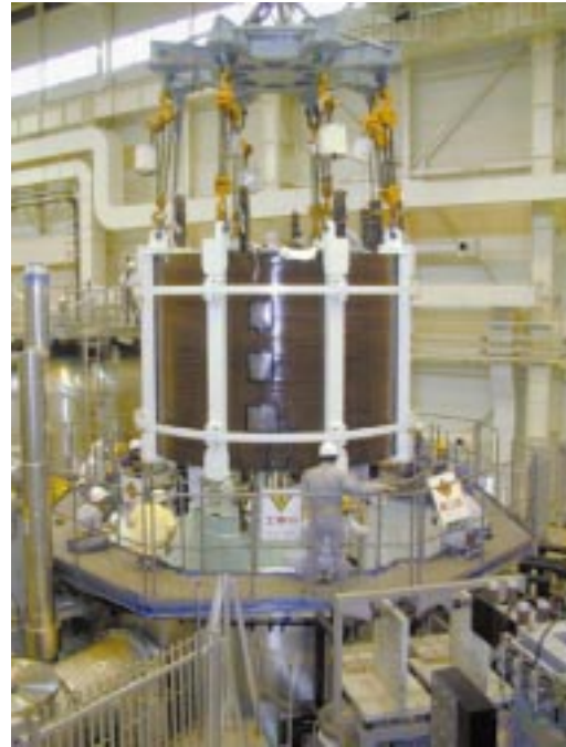
Figure 5. Central solenoid model coil facility, showing outer coil module insertion into the cryostat.
